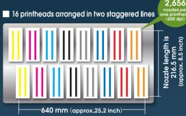
Tiger features 16 printheads (each line has 8 printheads) and allows a maximum high print speed of up to 385 m²/h\*. \* high speed (3 droplet size) mode 600 x 600 dpi, 1 pass. Bi; textile width ; 1.850 mr
