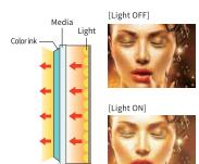
Single-layer printing looks faded when the illumination is on because too much light is transmitted.
