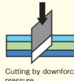
The blade edge is automatically and precisely controlled along contour cutting lines specified by the software. It is good for cardboard and foam board.
