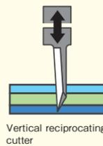
The blade cuts thick materials by a vertical reciprocating motion. It is ideal for foam or cardboard cutting. In addition, the blade is capable of cutting a range of material thicknesses, from thin to thick, by precisely controlling the blade edge direction. (Before cutting, please place a felt mat on the cutting table under the material to hold it in place.)
