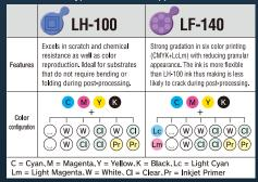
\*\*As ink flexibility of LF-140 ink varies according to the substrate to be printed, please be sure to test it beforehand \*\*LF-140 ink set does not include clear ink. You can use a combination with LH-100 clear ink.
