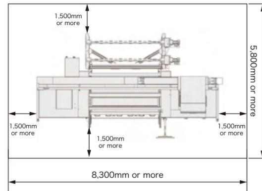
Entering within 1 meter of perimeter is extremely dangerous during the production
