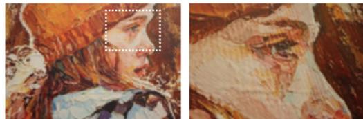
Automatically generates texture layering data from graphic information in RasterLink7. This process applies UV ink in layers to produce textured effects, with thicker layers resulting in more pronounced bumps and dips.
