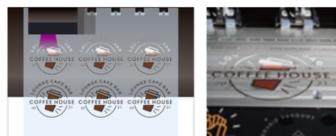
Designs are printed on special glued film, then application sheet is pasted on the film automatically.
