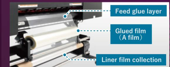
Automatically takes-up the UV-DTF film liner paper at the back of the machine. The liner paper is rolled precisely at the printer's feeding speed, ensuring stable printing.
