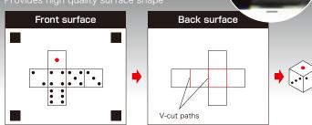
After detecting the printed marks and media edge, the back side is cut.
