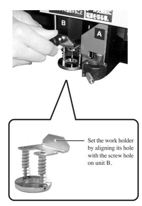
Set the work holder to unit B and tighten the screw.
