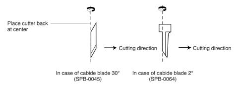
In pattern B, the tool is installed with tilted. Pattern B has to be adjusted so that horizontal lines and vertical lines are arranged in a straight line respectively along X- and Y-axes.
