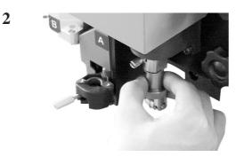
Insert the pin of unit C into the marking roller while fitting the pin in the groove on the roller.
