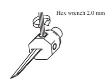
Push in the blade all the way into the cutter holder.
