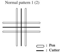
11  $(ADJUST > \theta 2/3)$ CUTTER  $\theta$  \*\*.\*\* > PATTERN No. \*1 > TEST PATTERN --->
