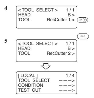
Select the tool to be used. RecCutter 1 RecCutter 2
