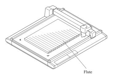
Place the corrugated board in such a way that its flutes are in parallel to the Y-axis of this device. To set a marking pressure in terms of the Y-axis direction, specify how far the pressure is reduced from the pressure value designated in the [CUTTING CONDITIONS]. See page 2.23.
