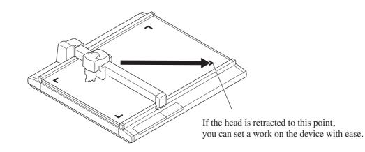
• If the "VIEW" (see page 1.29) is specified, the head will automatically move to the retracting point after the completion of cutting (plotting). This omits the execution of the "VIEW" function.
