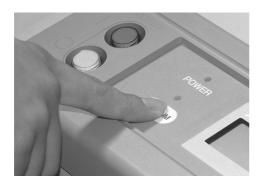
**Press the** (vacuum) **key.** The VACUUM lamp lights up (in green).
