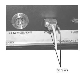
Insert the other end of the signal wire cable for the blower into the connector on the blower unit.
