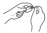
10. Insert the clean wiper with holding both projections at the tips of wiper.
