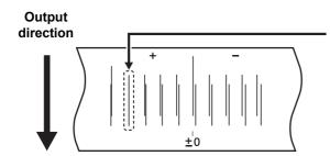
The dots at the fourth position counted from the zero position in the positive direction form a straight line. In this case, the dot position correction value is 4.0.
