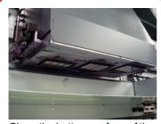
Clean the bottom surface of the slider and around the head with a cleaning stick.
