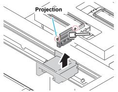
Further, in the cases as explained below, replace the wiper with the new one in accordance with "Replacing the wiper" on Chapter 4 of the Operation Manual.
