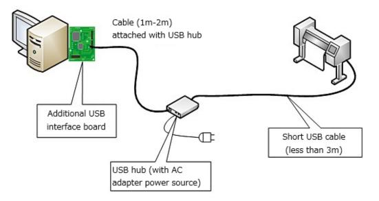
7 There may be incompatible USB2.0 cables in the market. Use recommended USB cable (OPT-J0137: USB2.0 cable (5m)) which is tested.
