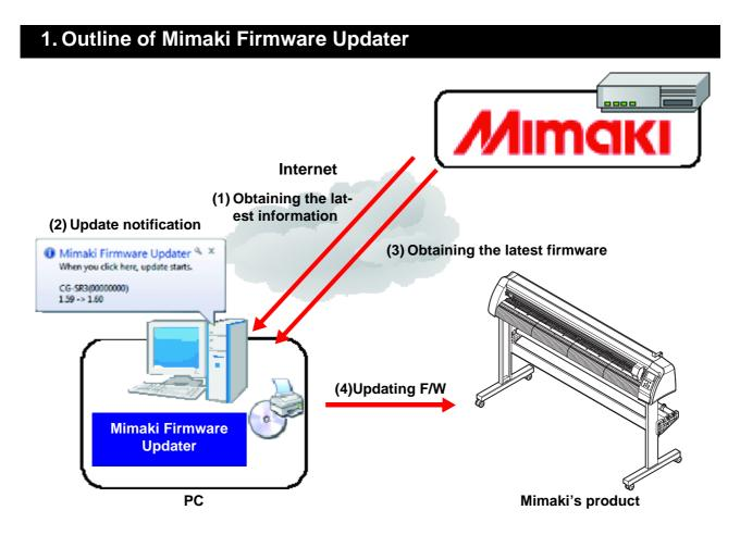
Mimaki Firmware Updater is the software that downloads the most recent firmware for the Mimaki products connected to PC form Web server, and updates the firmware.
