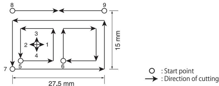
1. Select a tool to be used for test cut using the [TOOL SELECT] function. Call up the first page of the LOCAL menu to the screen. (P. 2-22)
