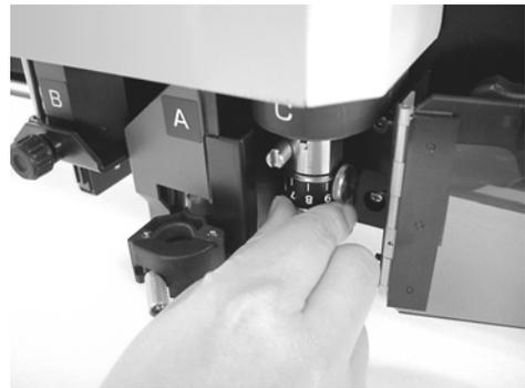
**3. Tighten the stopper screw with the screwdriver supplied with the device as an accessory.**
