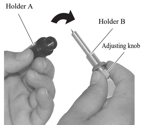
**3. Replace the blade tip with a new one using a pair of tweezers.**
