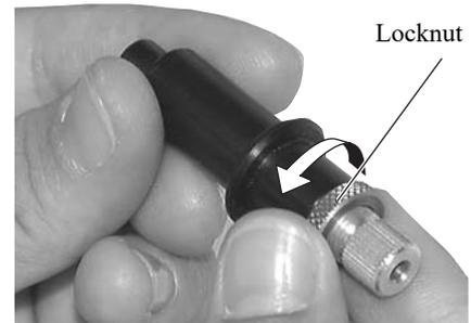
**2. Turning the adjusting knob counterclockwise, draw out the holder B from the holder A.**
