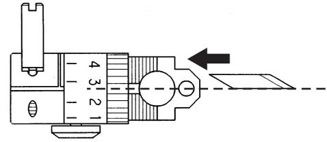
**3. Tighten the cutter stopper.**
