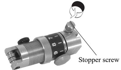
**2. Insert the pin of unit C into the tangential cutter while fitting the pin in the groove on the cutter.**
