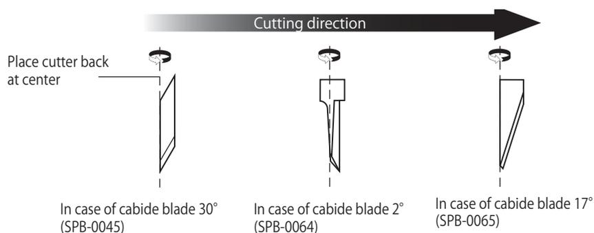
In pattern B, the tool is installed with tilted. Pattern B has to be adjusted so that horizontal lines and vertical lines are arranged in a straight line respectively along X- and Y-axes.
