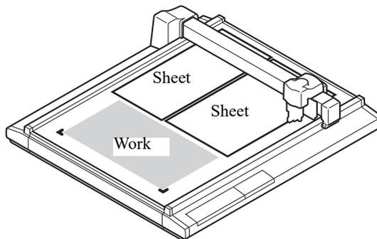
1. Place a work on the cutting panel.
