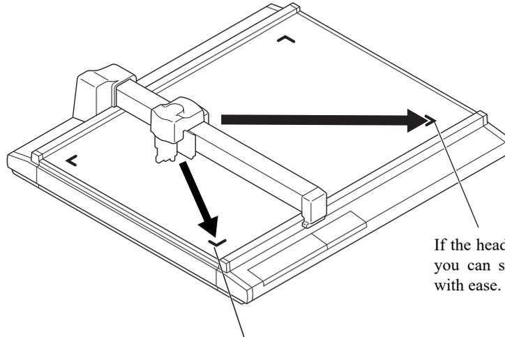
If the head is retracted to this point, you can set a work on the device with ease.
