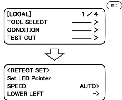
**3. Move and align the light pointer on the center of the TP1 vertical line precisely with jog key. In the case of square mark, move to around the center.**
