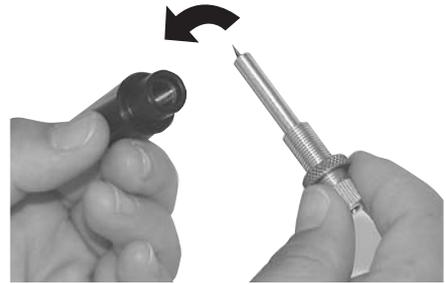
5. **Tighten the locknut.**
