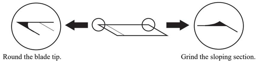
Gently rub the blade tip with the hand lapper while checking how far it is ground.
