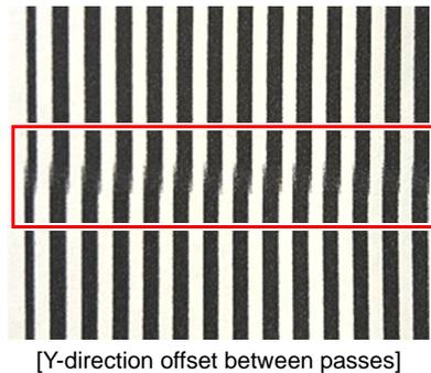
As this function reduces the scan speed, the productivity of the printer is reduced in exchange for improved image quality.
