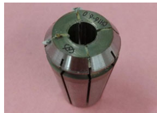
Debris accumulated in the chuck grooves
