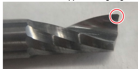
End mill with chipped cutting edge
