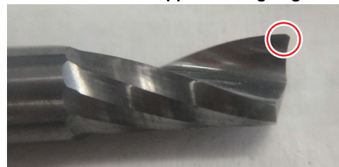
End mill with chipped cutting edge
