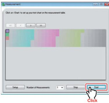
9 Pressing the button on the measurement device, align the target chart with the part indicated on the screen (the upper left).
