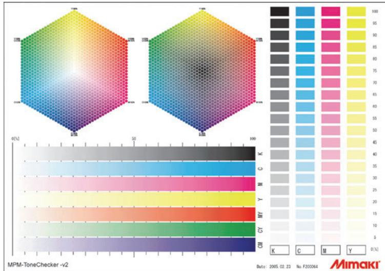
The variable dots spray the dots of 3 sizes (Small, Middle and Large) and make the gradation smooth. The optimum parameters are provided to make the gradation smooth according to the ink set you use.
