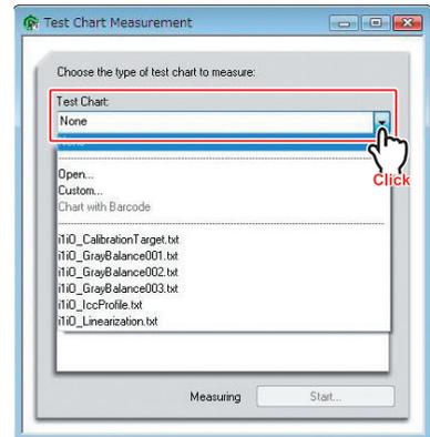
Eye-One iO chart is displayed. Select the chart having the name of element for color measurement. (In case of adjusting the linearization, select [i1iO\_Linearization.txt].)
